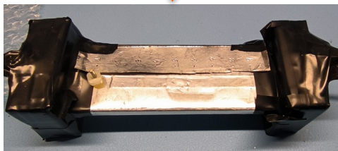
PST bar with a SiPM board at each end
