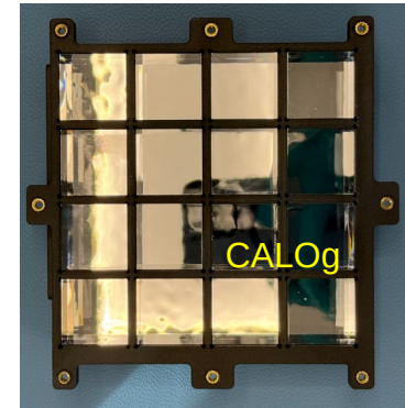
CALOg board (SiPMs 1x1, 3x3, 6x6 mm 2 )
