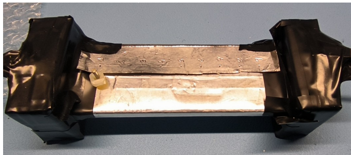
PST bar 1.0 cm, Sr-90 on top, SiPM at each end.
