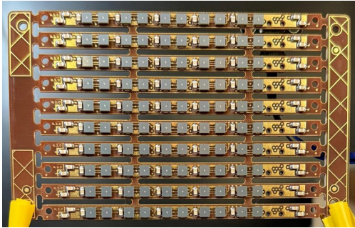
ACS board (SiPMs 3x3 mm 2 )
