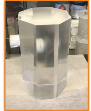
NaI-33 after cut and polishing
