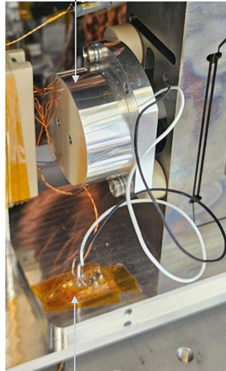
Low-noise voltage buffer made with MELF resistors
