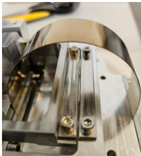
Thermal treatment to get an almost-zero TEC
