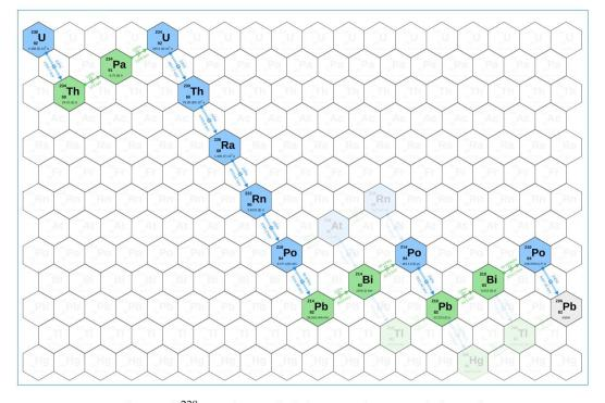
**Figure 6.28:** Decay chain of <sup>238</sup>U. The probabilities and types of decay between isotopes are shown (blue for alpha and green for beta decays). The half-life of each element is also indicated. The energies correspond to the Q-values of the decays. Figure taken from [277]
