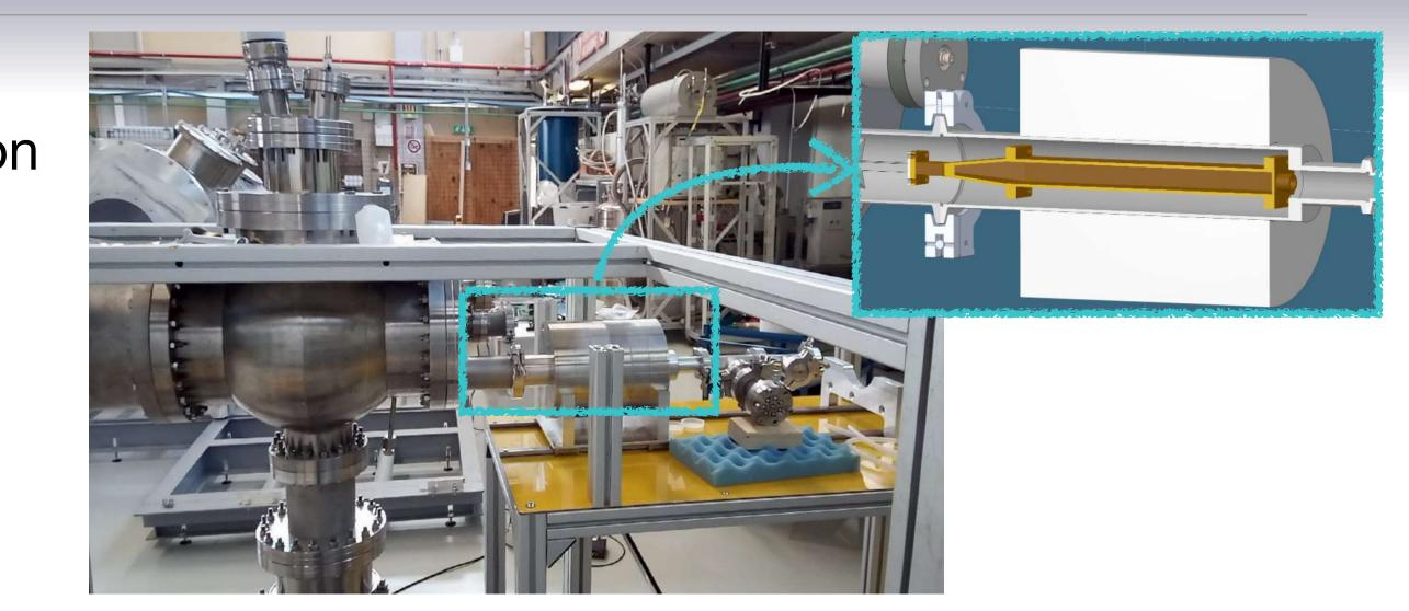
Electron gun setup for calibration
