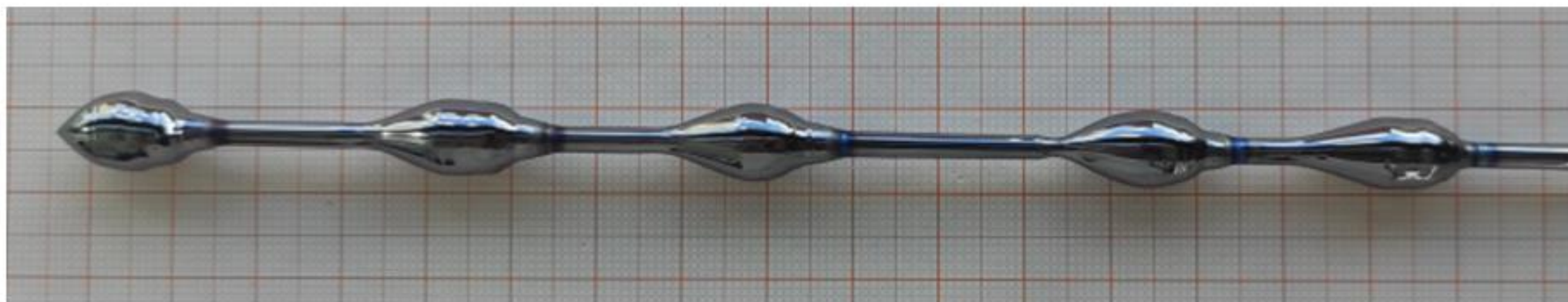
As-grown Si-fiber with nodes of different shapes
