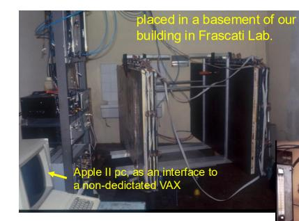
The tracking telescope was made of 1 m long NUSEX-like streamer tubes (~1 cm<sup>2</sup> cross section) equipped with 2-dim readout, oriented to look for muons at high zenith angle (to increase average muon energy)
