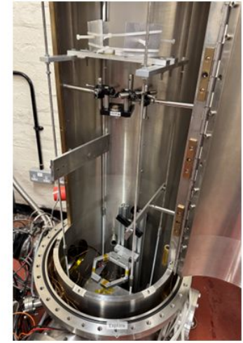
Stress corrosion vacuum setup
