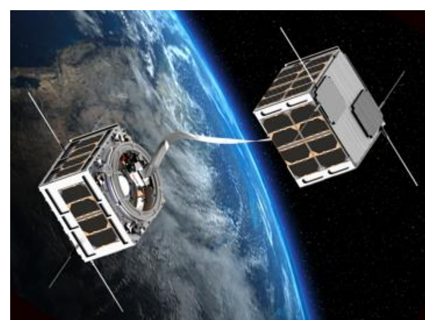
Figure 2. the Deorbit Kit concept (courtesy of E.T.PACK-F, www.etpack.eu )
