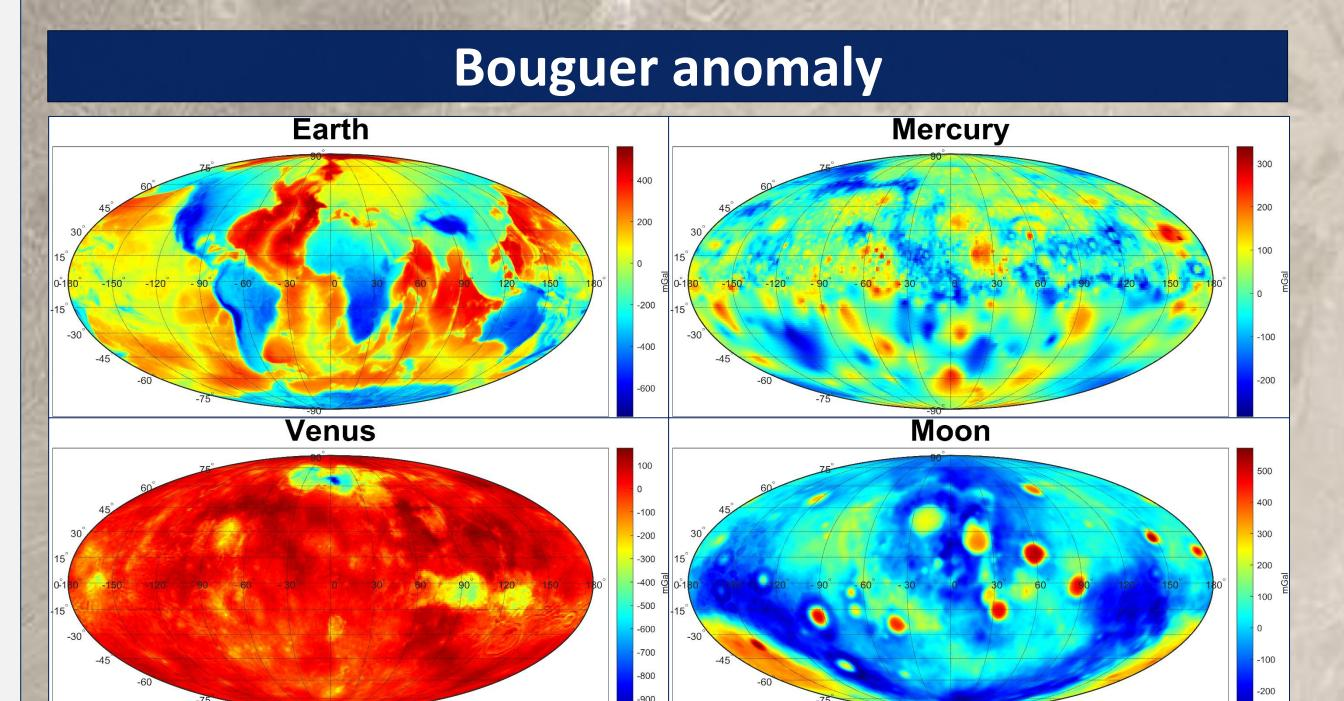
This results in two quantities to constrain the interiors: from the gravitational acceleration (i.e., Free-Air anomaly) the topography contribution can be subtracted, via **Bouguer correction**, while from the gravity spectrum, it is possible to analyse the **admittance** *Z*(*n*). In the following, the resulting equations:
