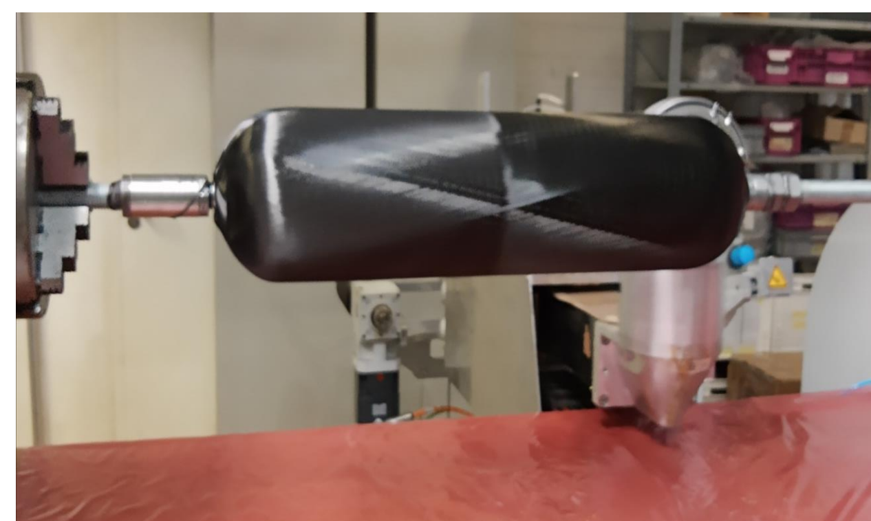
Fig. 4. Smart Propellant Tank carbon fiber filament winding in facilities of TUM (May 2024) – currently ongoing prototyping process.
