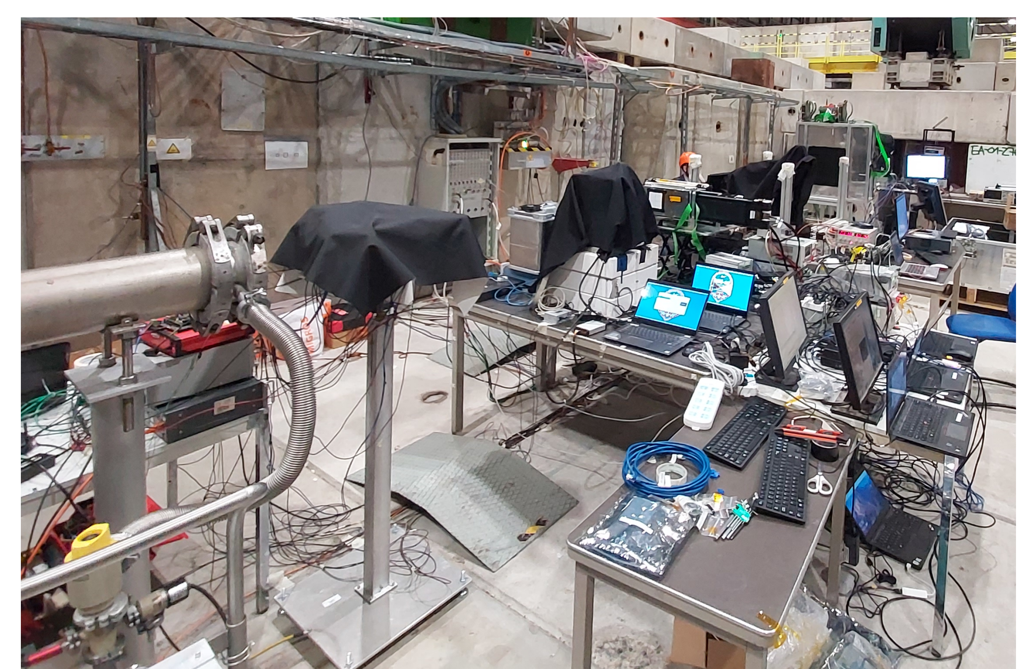
Figure: Detectors set-up along the CERN SPS beamline during the November 2022 beam test.
