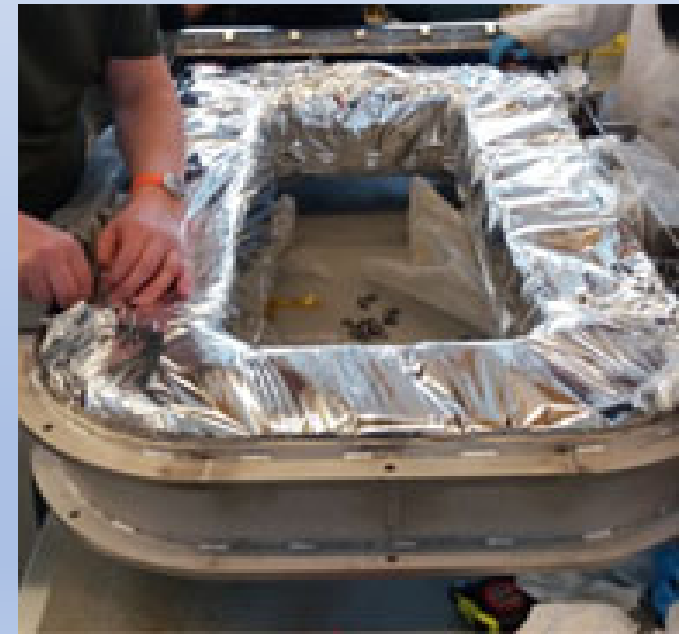
Packed with multi-layer thermal insulation
