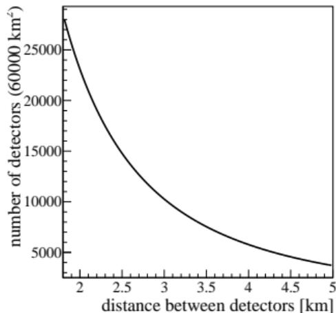
Spacing between detectors cannot be larger than about 2-2.5 km to reach 100% efficiency at 10-30 EeV
