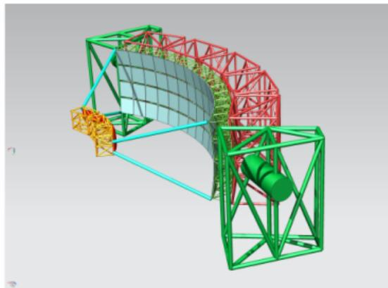
**Figure 7:** Proposed optics for *Trinity* based on the MACHETE optics. The primary mirror is composed of 68, 1 m<sup>2</sup> mirrors. the focal plane (red curved surface) is populated with 3,300 pixels each consisting of a solid non-imaging light concentrator coupled to an SiPM. The field of view covered by one telescope is 5° × 60°.
