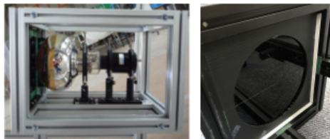
8 in. PMT with UV transmitting filter.
