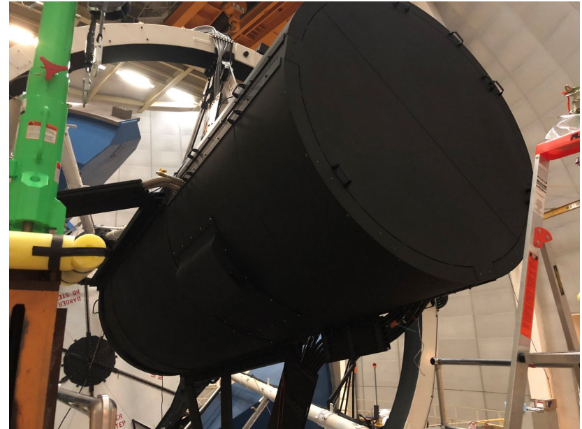
Focal plane inside its environmental enclosure
